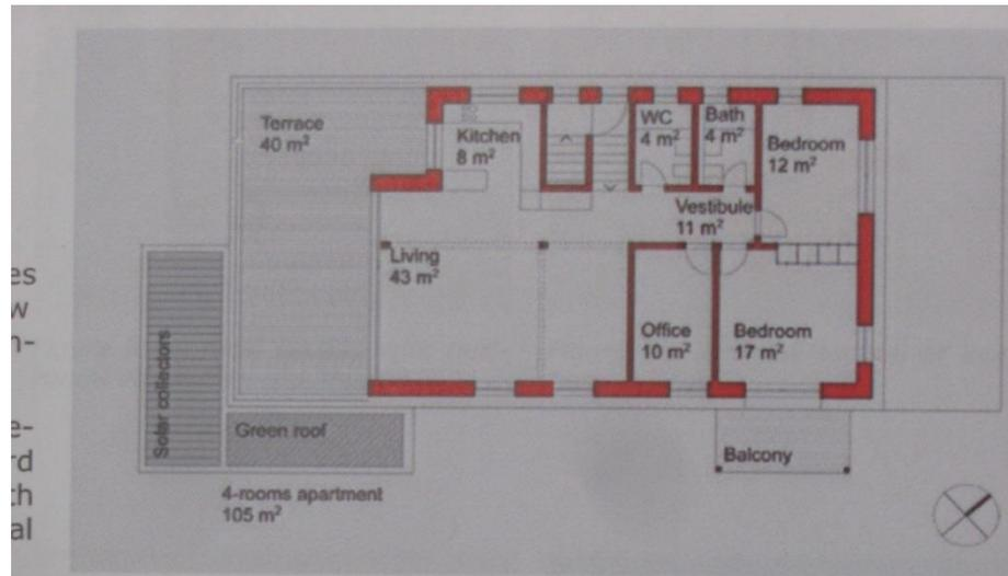
Figure 6: Floor plan of added penthouse apartment
