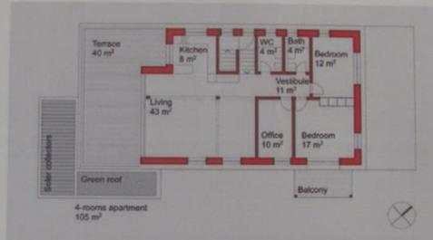
Figure 6: Floor plan of added penthouse apartment
