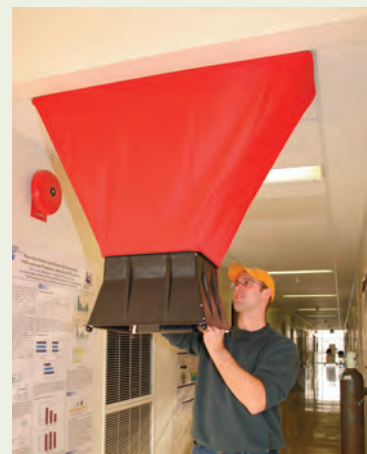
Checking air flow in HVAC system. "Continuous commissioning" is one of Penn State's strategies to maximize building energy efficiency.
